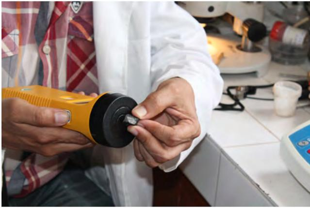
Figure 5 – A. Ibhi measuring the magnetic susceptibility on a fragment of Igdi meteorite at the Ibn Zohr University.
