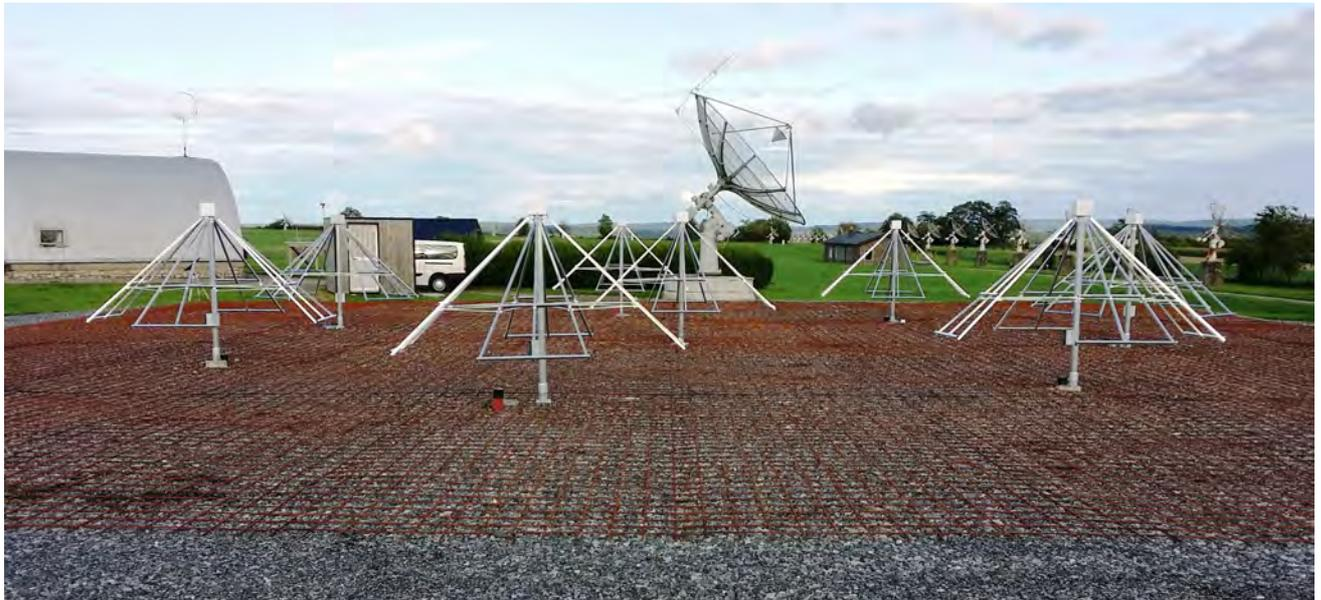
Figure 5 – General view of SPADE array field in HuRAS. Behind the SPADE antennas, the 6 m-dish and its piggy-backing log-periodic antennas (used by the HSRs, ARCAS, and CALLISTO instruments) can be seen.
