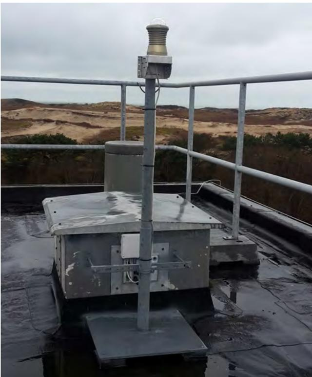
Figure 1 – FRIPON camera installed at the European Space Agency’s center ESTEC, in Noordwijk, the Netherlands.
