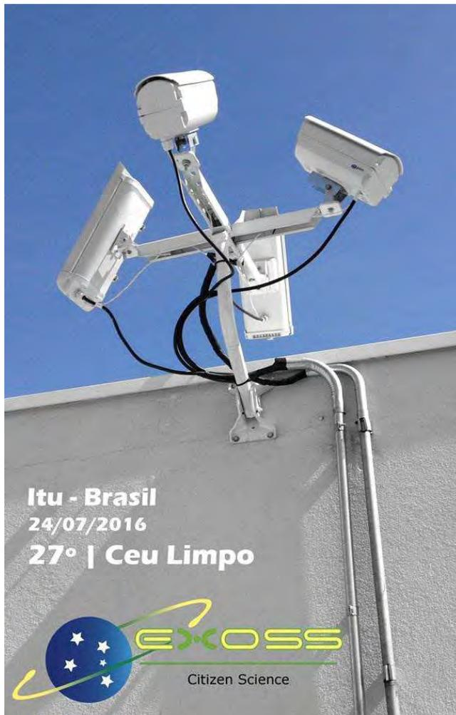
Figure 2 – Four cameras setup of the EXOSS station in Itu, in São Paulo state.
