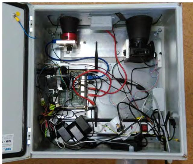
Figure 2 – Inner view of the prototype of the planned optical unit, including a video and DSLR camera, cooling, sensors and an SBC.
