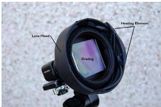
Figure 1 – Usual configuration for video meteor spectroscopy.
