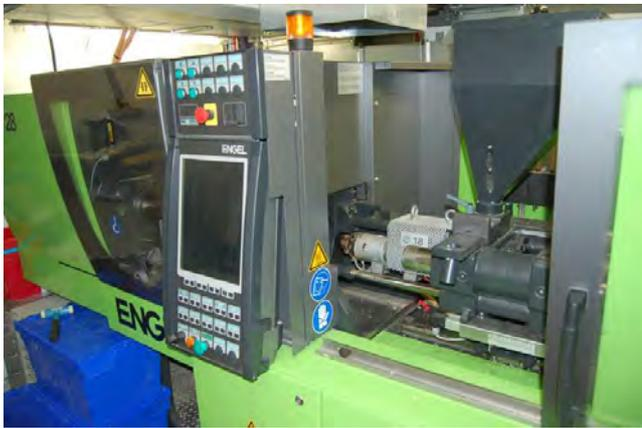
Figure 3 – Victory 28 injection moulding machine.
