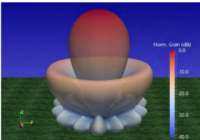
Figure 3 – 3D visualization of SPADE array pattern simulation in 50 MHz for a circular distribution of antennas around a central one.
