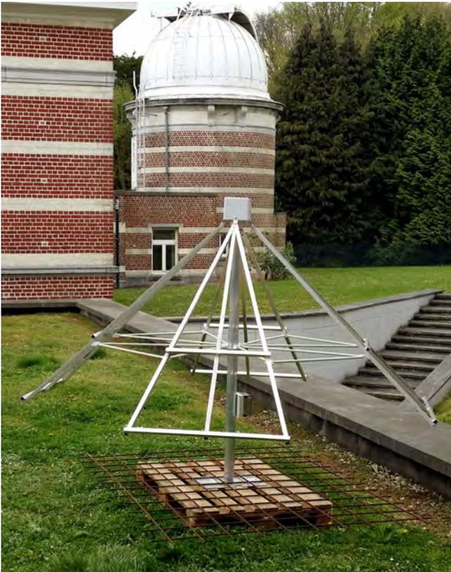
Figure 2 – Wide-band antenna selected as SPADE array element installed at the Royal Observatory of Belgium during a testing period.
