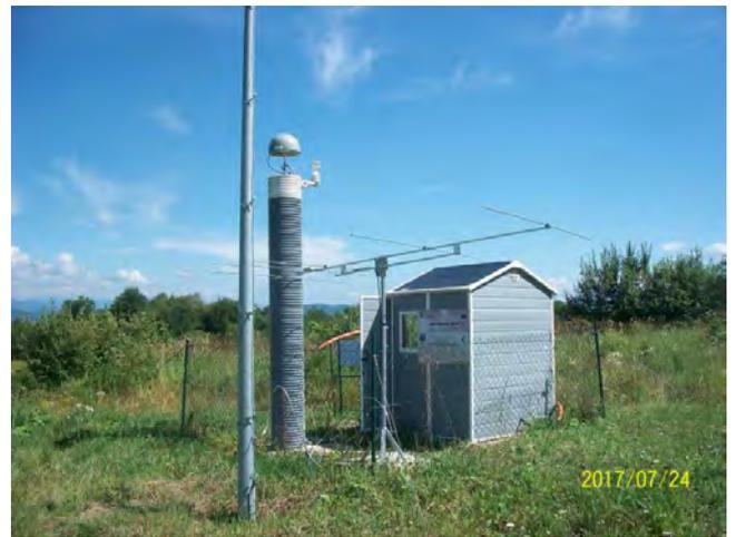
Figure 4 – Five-element Yagi transmitting antenna at Kolonica Observatory.
